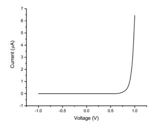
Fig S4 I-V trace for the charge tunable p-i-n diode showing rectification behavior at a temperature of 5.4 K.
