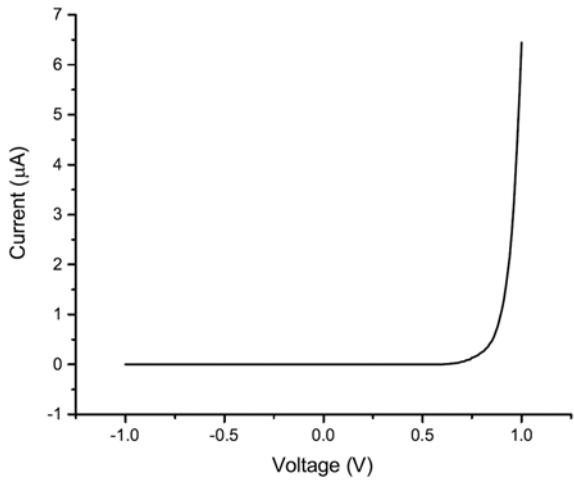
**Fig S4** I-V trace for the charge tunable p-i-n diode showing rectification behavior at a temperature of 5.4 K.
