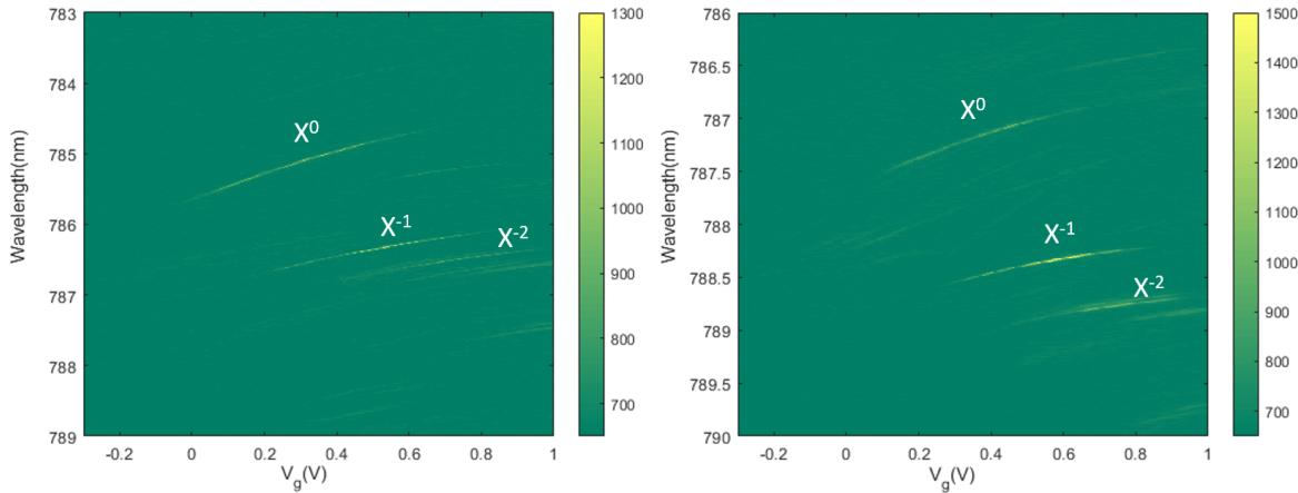
**Fig S5** Charge plateaus for two different QDs at a temperature of 6 K while this QD is being excited by a non-resonant 632.8 nm laser.
