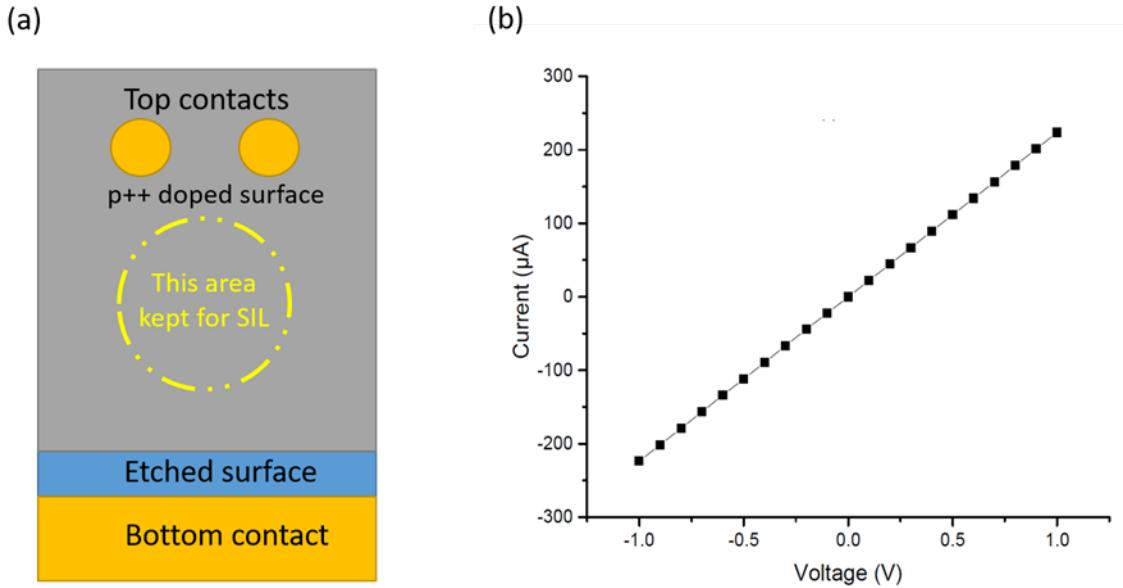
**Fig S3** (a) Top view of the fabricated p-i-n diode. (b) I-V trace for the two top contacts on the p++ doped surface showing Ohmic behavior at 5.4 K.
