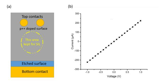
**Fig S3** (a) Top view of the fabricated p-i-n diode. (b) I-V trace for the two top contacts on the p++ doped surface showing Ohmic behavior at 5.4 K.
