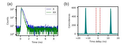
**Fig S6** Decay dynamics of a QD in a p-i-n diode structure at a temperature of 5 K under resonant two-photonexcitation. (a) Lifetime trace of the XX and X photons, with lifetimes of 116(2) ps and 238(3) ps, respectively. (b) Example of a coincidence histogram between the XX and X photons in the HV measurement basis. The red dashed lines indicate the time-bin of 2 ns in which the coincidences are summed up to calculate the peak areas.
