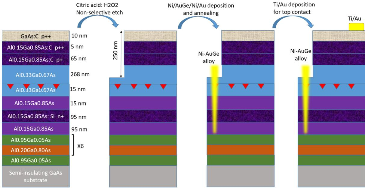
**Fig S2** Fabrication steps for a charge tunable diode: Pristine sample structure to the fabricated contacts for the n- and p- sides using lithography, non-selective wet etching, metal deposition and thermal treatment.
